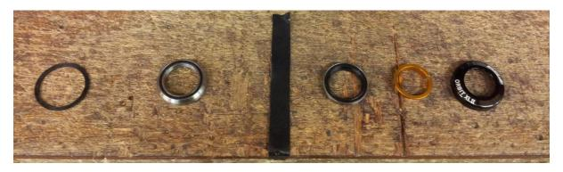
Starting with the lower headset cup make sure the cup is clean and free from any sticky tape, dust or card shavings
