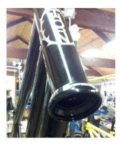
Then insert the thicker of the two cartridge bearings
