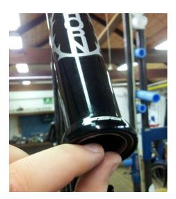
Then tuck the black rubber/plastic shield into the grove in the lower cup, this will hold the bearing in
