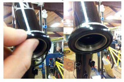
With the upper headset cup make sure the cup is clean and free from any sticky tape, dust or card shavings
